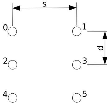
**Figure 1.** Eyelet numbering and dimensions for  $N = 3$ .
