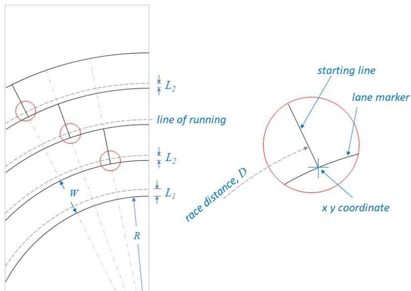
**Figure 2.** Inset showing staggered starting line locations.
