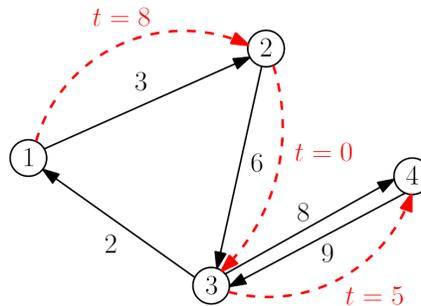
**Figure 1.** Illustration of sample input. Scheduled trips are depicted by dashed red lines with their respective start times. The optimal solution is to have one driver complete the trip from 2 to 3 at time 0, then travel to location 1 arriving at time 8, and then complete the trip from 1 to 2. The second driver can complete the trip from 3 to 4.
